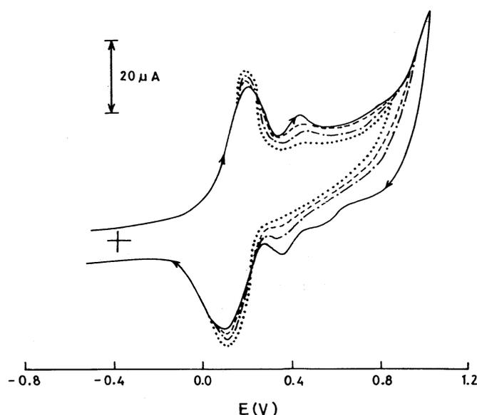
**Figure 3.** Effect of  $pH$  on cyclic voltammogram:  $pH = 4.5$  (—);  $pH = 3.9$  (- - -);  $pH = 3.3$  (- · -);  $pH = 2.8$  (·····) in MeCN solution.
