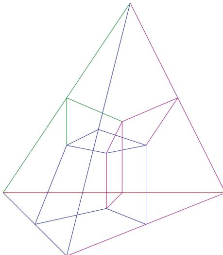
**Figure 5.** Decomposition of a tetrahedron into four hexahedrons.
