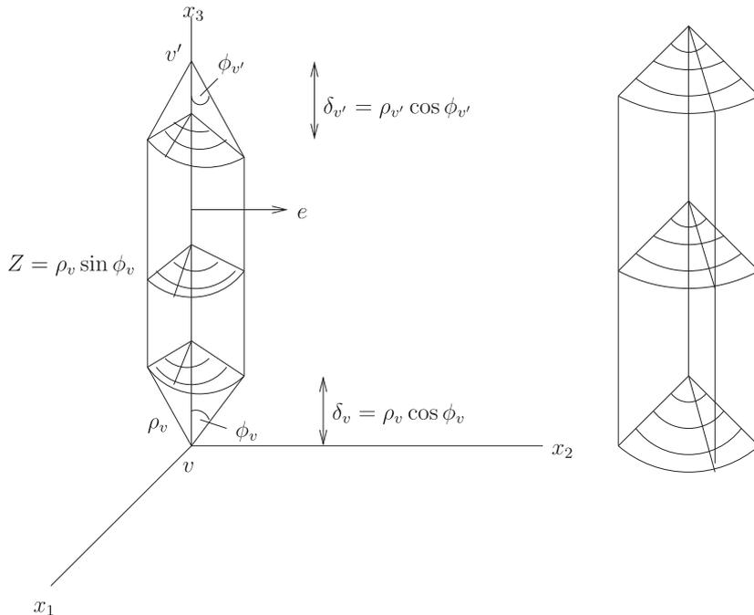
**Figure 10.** Geometrical mesh imposed on  $\Omega^e$ .
