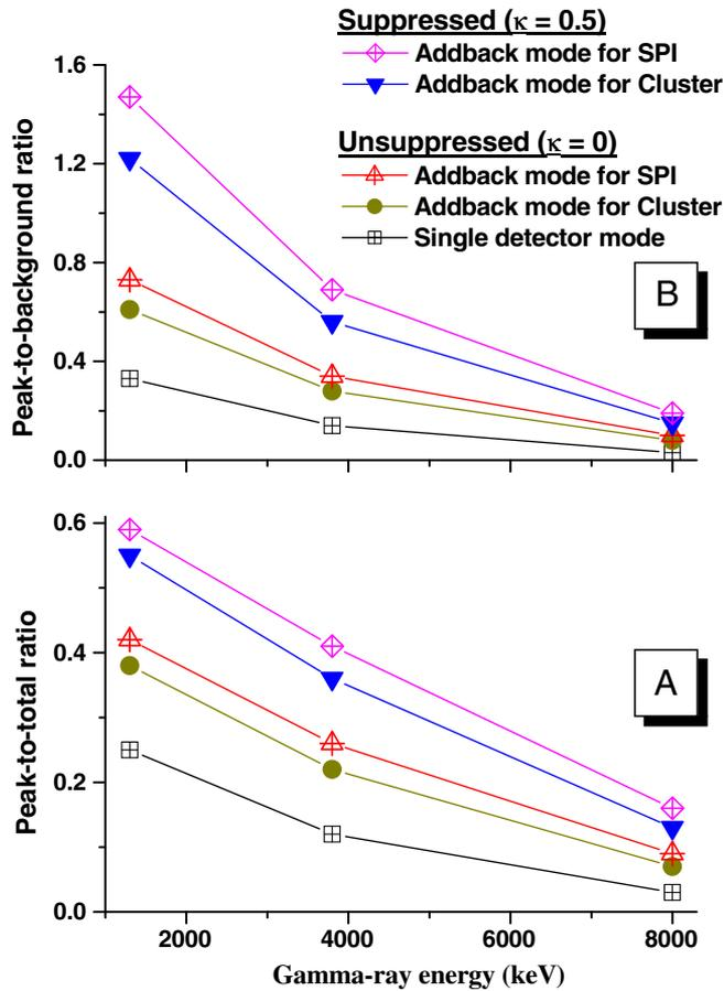
**Figure 2.** PT and PB ratios are plotted as a function of  $\gamma$ -ray energy in (A) and (B), respectively. Results are shown for various modes of operation and suppression cases for the cluster detector and SPI spectrometer.
