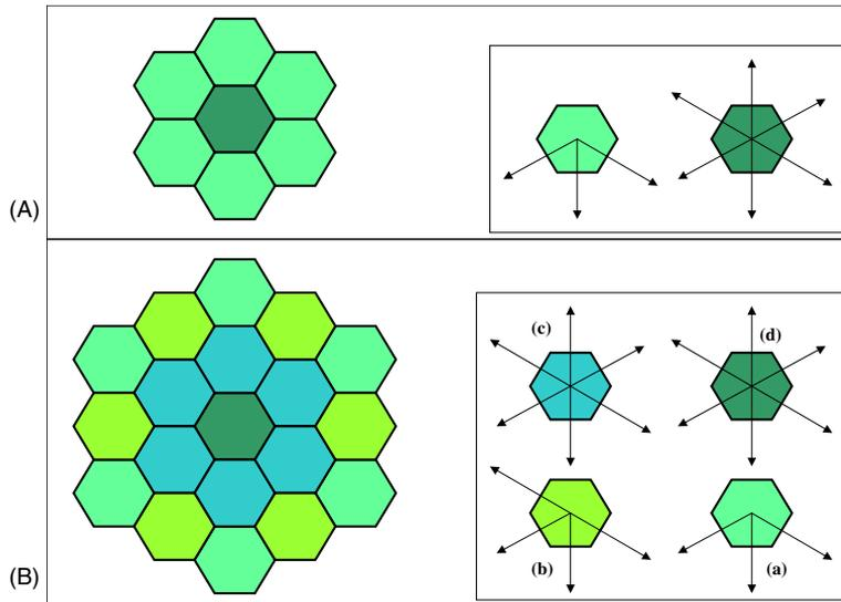
**Figure 1.** The cluster detector and the SPI spectrometer are schematically shown in figures (A) and (B), respectively. Inset shows possible  $\gamma$ -ray scatterings from different groups of detector modules to adjacent modules.
