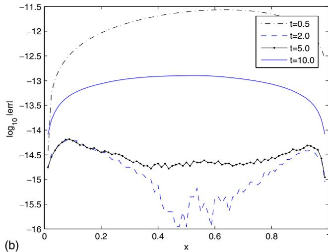
**Figure 4.** Log 10 of the absolute error in Example 3 with  $\alpha = 6$  at different time levels. (a)  $k = 0.0001$  and  $N = 20$ , (b)  $k = 0.00005$  and  $N = 80$ .
