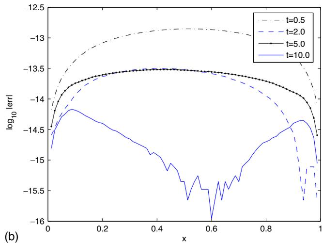
**Figure 5.** Log 10 of the absolute error in Example 4 with  $a = 0.2$  at different time levels. (a)  $k = 0.0001$  and  $N = 20$ , (b)  $k = 0.00005$  and  $N = 80$ .
