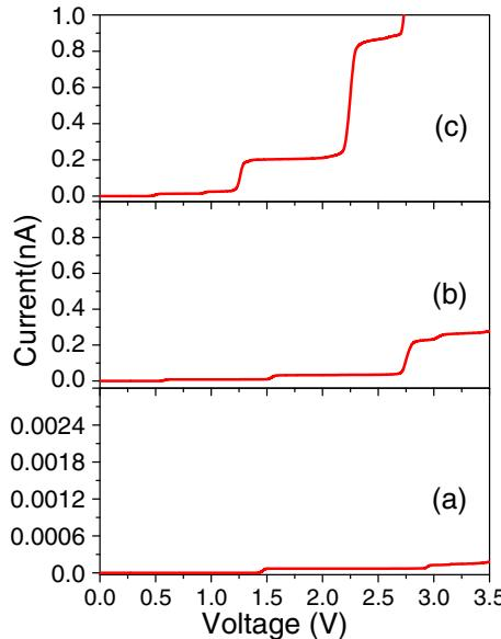
**Figure 3.** (a)–(c) panels show the  $I$ – $V$  characteristics of (10,0) BCN alloy nanotube for 20, 50 and 80% concentration of C atoms, respectively.
