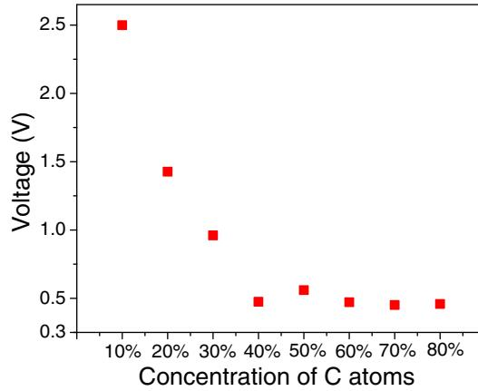
**Figure 4.** The corresponding voltage in the first step of the  $I$ - $V$  characteristics. The horizontal axis corresponds to 10, 20, 30, 40, 50, 60, 70 and 80% concentration of C atoms respectively for (10,0) BCN alloy nanotube.
