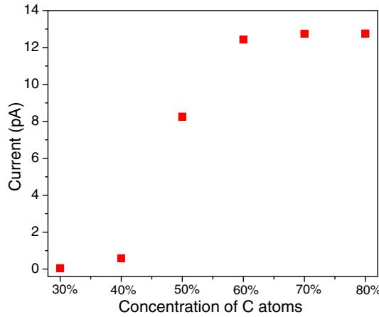
**Figure 5.** The corresponding current in the first step of the  $I$ - $V$  characteristics. The horizontal axis corresponds to 30, 40, 50, 60, 70 and 80% concentration of C atoms respectively for (10,0) BCN alloy nanotube.
