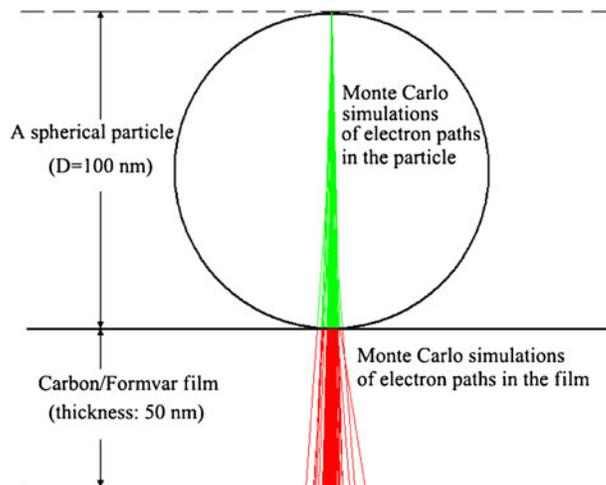
**Figure 1.** Electron paths obtained by Monte Carlo calculation under TEM-EDX measurement condition for a spherical particle sitting on carbon/formvar film (adapted from Geng *et al* [8]).
