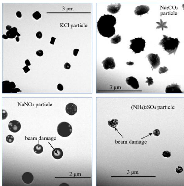
**Figure 2.** TEM images of KCl, Na<sub>2</sub>CO<sub>3</sub>, NaNO<sub>3</sub> and (NH<sub>4</sub>)<sub>2</sub>SO<sub>4</sub> standard particles (adapted from Geng *et al* [8]).
