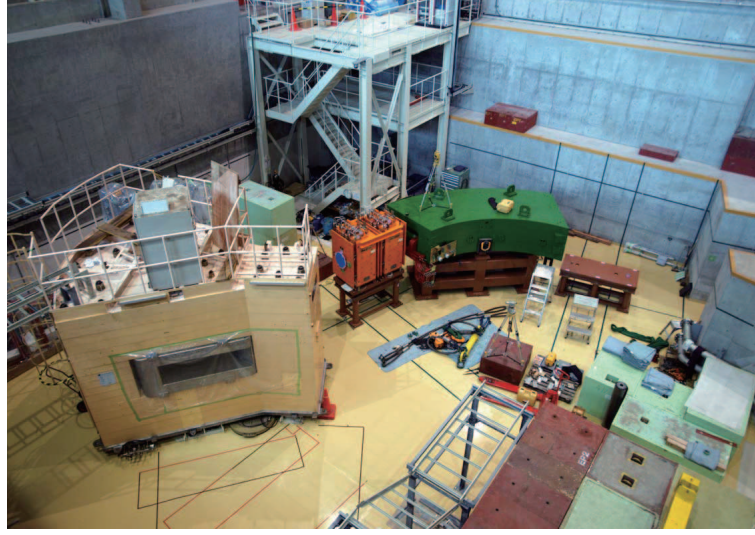
Figure 4. A picture of K1.8 area in the hadron experimental hall of J-PARC, in which the beam line spectrometer and the SKS spectrometer are being installed.
