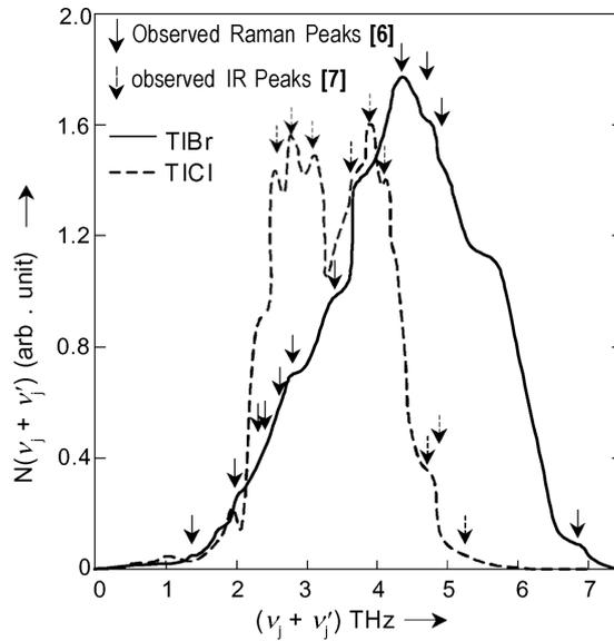
Figure 3. Phonon density of state curves for TlBr and TlCl.
