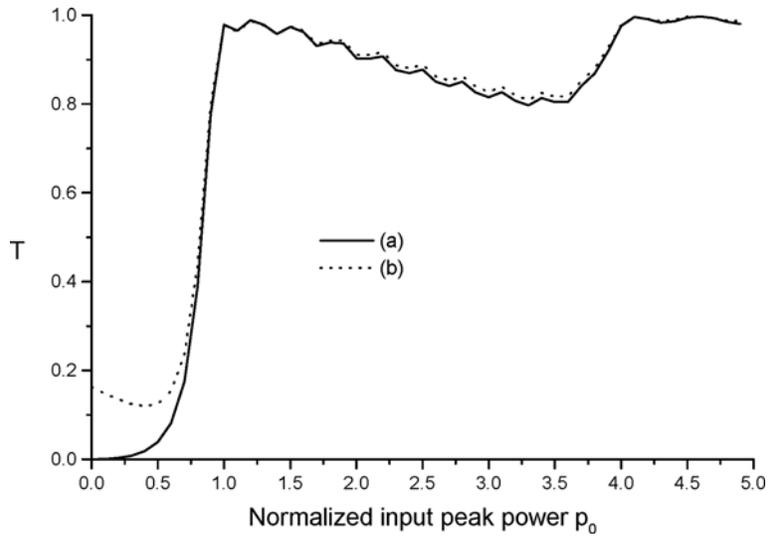
**Figure 1.** Plot of the transmission coefficient as a function of the normalized input peak power for soliton of pulse width 10 fs with  $\kappa_0 = 0.1$ . Curve (a) corresponds to the case without any perturbative effects including IMD and curve (b) corresponds to the case when only IMD is taken into account.
