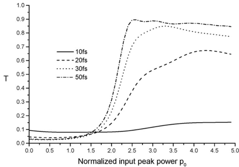
**Figure 3.** Plot of the transmission coefficient as a function of the normalized input peak power for solitons of various pulse widths  $T_0$ . Here the coupling coefficient  $\kappa_0 = 0.5$ .
