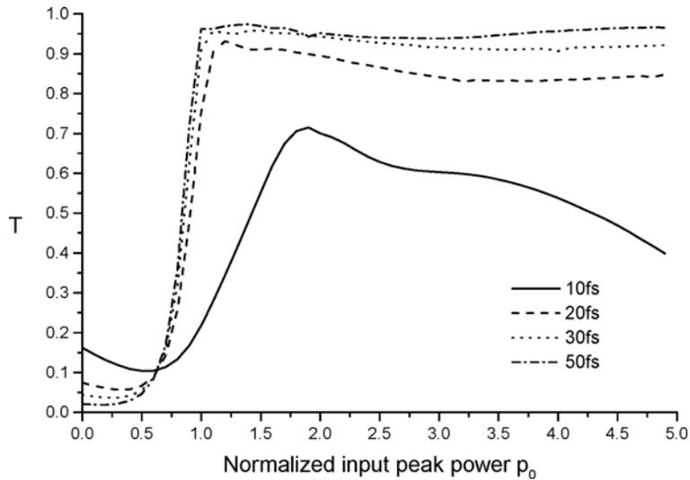
**Figure 2.** Plot of the transmission coefficient as a function of the normalized input peak power for solitons of various pulse widths  $T_0$ . Here the coupling coefficient  $\kappa_0 = 0.1$ .
