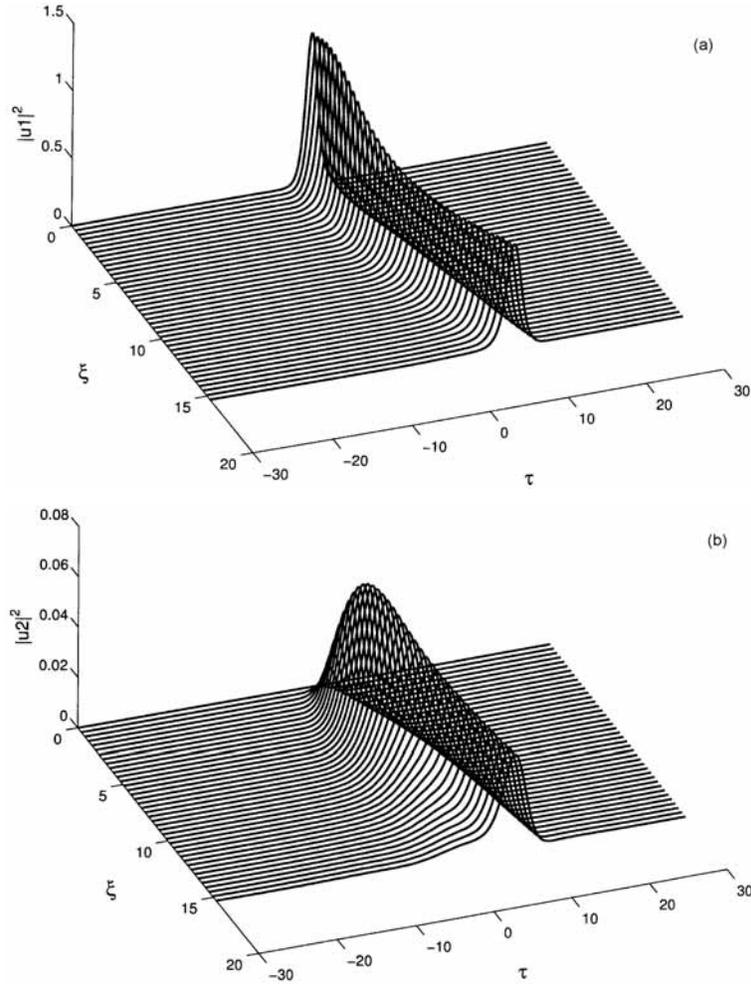
**Figure 6.** (a) Evolution of a 20 fs soliton pulse inside the coupler in core 1 (parallel state of the coupler) with  $\kappa_0 = 0.1$ . (b) Evolution of a small soliton with some radiation leaked into core 2 (crossed state of the coupler) with  $\kappa_0 = 0.1$ .
