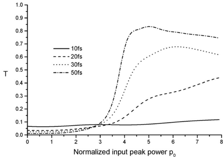
**Figure 4.** Plot of the transmission coefficient as a function of the normalized input peak power for solitons of various pulse widths  $T_0$ . Here the coupling coefficient  $\kappa_0 = 1.0$ .
