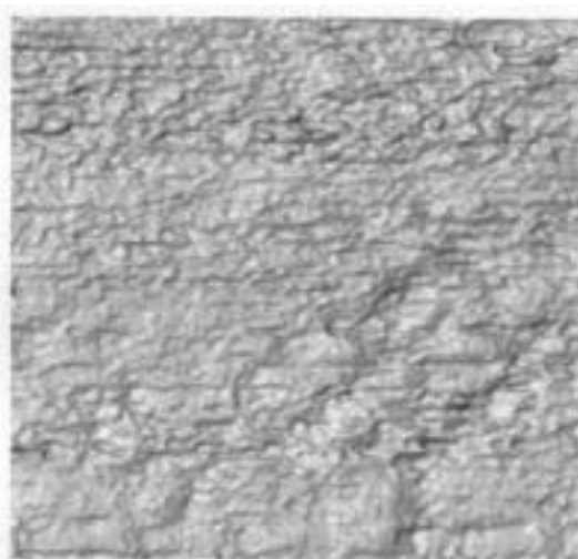
Figure 6. The scanning tunnel microscopy of the center of the vanadium sample with a thickness of 0.29 mm. The irradiation of the sample was done by the pulse of deuterium plasma at a distance of 10 mm from the anode of plasma focus. Size of the area is 1.2 \times 1.2 \mu\text{m} .
