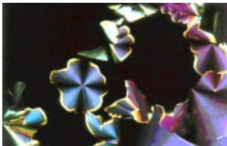
**Figure 1.** Optical photomicrograph of the hexagonal columnar phase developing from the isotropic liquid, compound **2**, 79.0°C.
