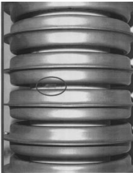
Figure 6. Crack in column support post.
