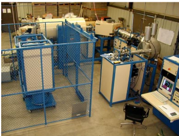
Figure 3. The high throughput carbon AMS system equipped with 134 sample, multi-cathode source of negative ions by cesium sputtering (134 MC-SNICS). This system is presently in operation at the Center for Applied Isotope Studies, University of Georgia, USA.
