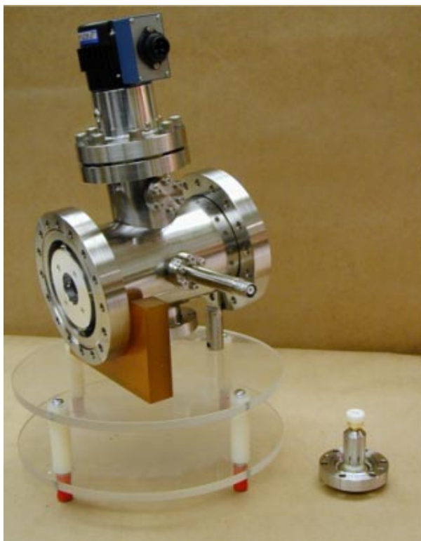
Figure 4. The low current beam profile monitor (LCBPM) which is under development for the cross-sectional measurement of ion and electron beams from the particle/s to the microamp range.
