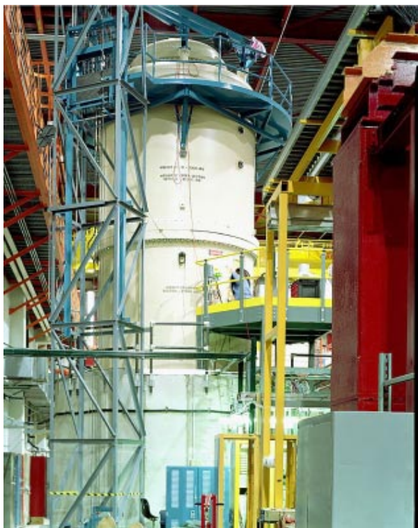
Figure 1. The 5UR Pelletron which is housed in a pressure vessel, 7.7 m high by 3.66 m in diameter. The column has two parallel acceleration tubes. The first tube allows the beam acceleration from the terminal electron gun. The second tube allows the beam deceleration to the terminal charge collector. (Photo courtesy of Fermi National Accelerator Laboratory.)
