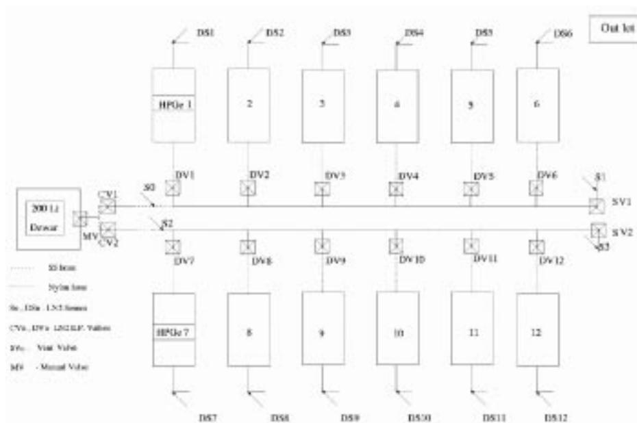
**Figure 1.** The schematic of the liquid nitrogen filling system.
