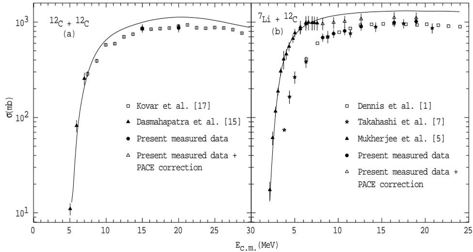
**Figure 2.** Fusion cross-sections for (a)  ${}^{12}\text{C} + {}^{12}\text{C}$  and (b)  ${}^7\text{Li} + {}^{12}\text{C}$  reactions. The solid curves are the optical model calculations obtained with parameters from (a) ref. [18] and (b) ref. [19].
