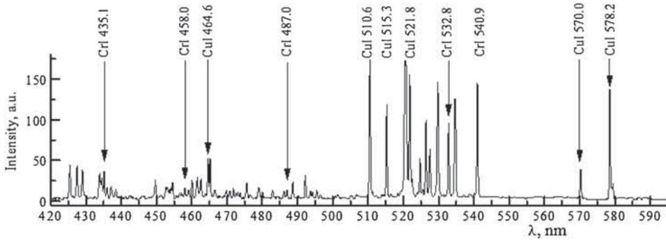
**Figure 11.** Emission spectrum of plasma of electric arc discharge between composite Cu-Cr-W electrodes in argon flow at 3.5 A.
