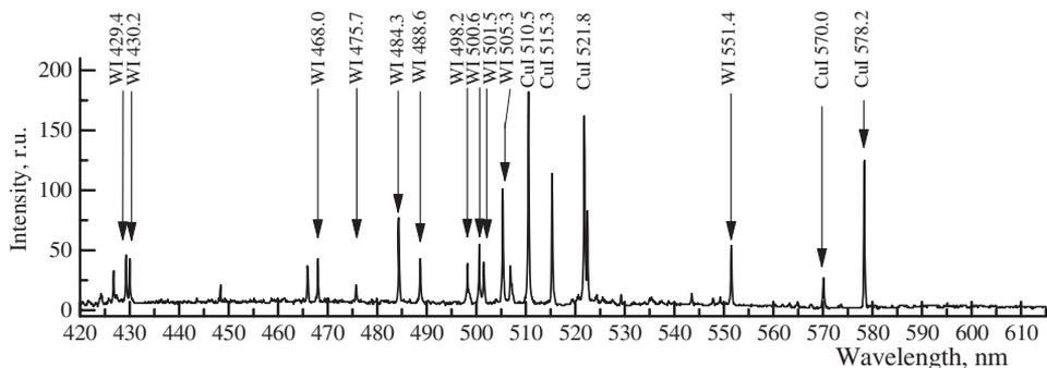
**Figure 7.** Emission spectrum of plasma of electric arc discharge between composite Cu–W electrodes in argon flow at 3.5 A.
