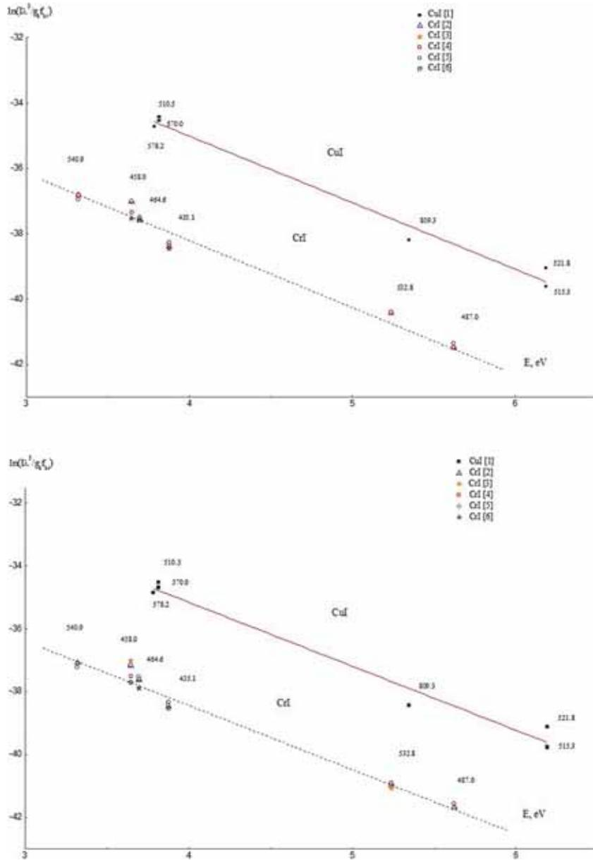
**Figure 13.** Boltzmann plots involving Cu I and Cr I spectral lines and selection of spectroscopic data of chrome spectral lines for the axial point (*left*) and at a distance of  $r = 1$  m (*right*) of the middle cross-section of plasma of free burning electric arc discharge between Cu–Cr–W electrodes at current of 3.5 A in argon flow. [1] Boretiskij (2011), [2] Ralchenko *et al.* (2010), [3] Kurucz & Bell (1995), [4] Younger *et al.* (1978), [5] Sobeck *et al.* (2007), [6] Wujec (1981).
