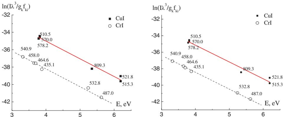
**Figure 14.** Boltzmann plots involving selected spectroscopic data of chrome spectral lines for the middle cross-section of plasma of free burning electric arc discharge between Cu–Cr–W electrodes for the axial point (*left*) and at a distance of  $r = 1$  mm (*right*) at 3.5 A in argon flow.
