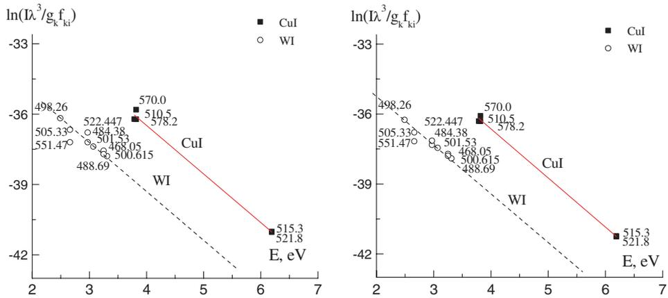
**Figure 9.** Boltzmann plots involving selected spectroscopic data of tungsten spectral lines of the middle cross-section of plasma of free burning electric arc discharge between Cu–W electrodes for the axial point (*left*) and at a distance of  $r = 0.9$  mm (*right*) at 3.5 A in argon flow.
