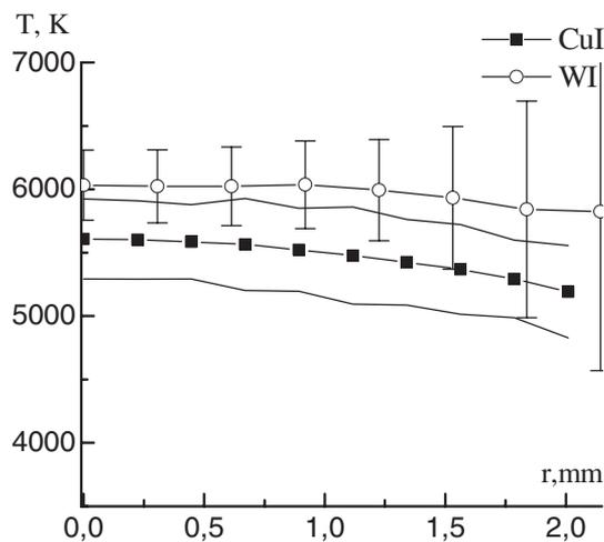
**Figure 10.** Radial distribution of the plasma temperature of electric arc discharge between Cu–W electrodes at 3.5 A in argon flow.
