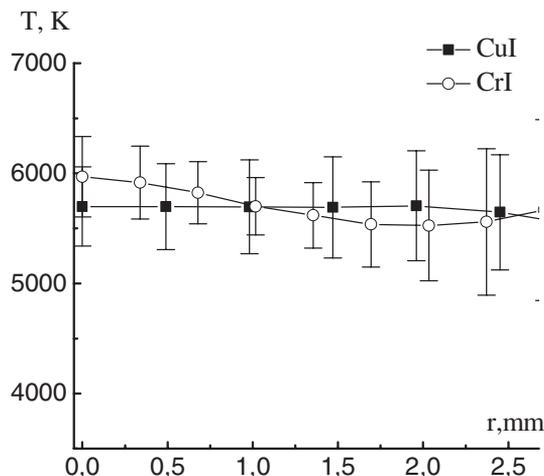
**Figure 15.** Radial distribution of the plasma temperature of electric arc discharge between Cu–Cr–W electrodes at 3.5 A in argon flow.
