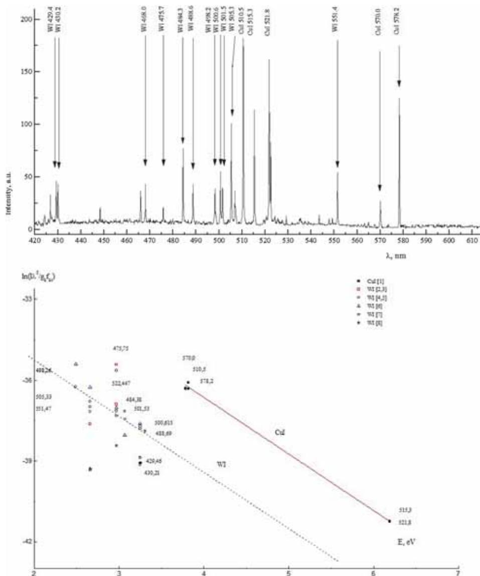
**Figure 8.** Boltzmann plots and selection of spectroscopic data of tungsten spectral lines in the middle cross-section of plasma of free burning electric arc discharge between Cu–W electrodes for the axial point (*left*) and at a distance of  $r = 0.9$  mm (*right*) at 3.5 A in argon flow. [1] Boretskij (2011), [2] Ralchenko *et al.* (2010), [3] Obbarius & Kock (1982), [4] Kurucz & Bell (1995), [5] Den Hartog *et al.* (1987), [6] Kirsanova (1969), [7] Kling & Kock (1999), [8] Thevenin (1989).
