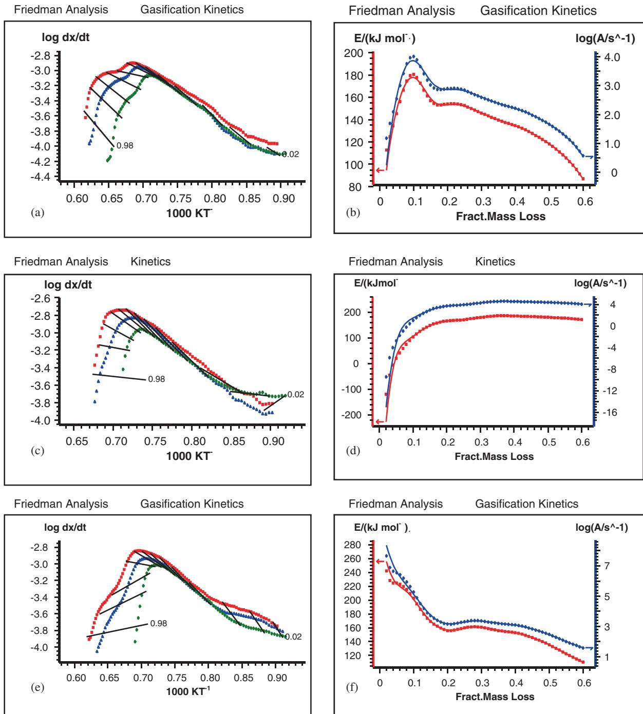
Figure 5. Freidman analysis and corresponding energy plot diagram of the Tirap (a, b), Tipong (c, d) and Bapung (e, f) samples.
