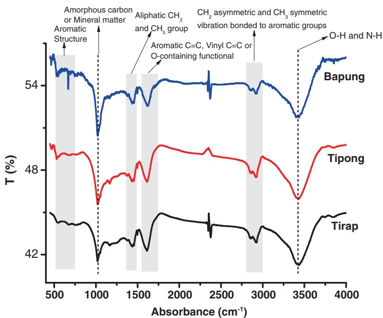
Figure 2. FT-IR spectra of coal samples.
