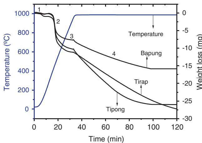
Figure 6. Isothermal analysis of the coal samples for their reactivity measurement.
