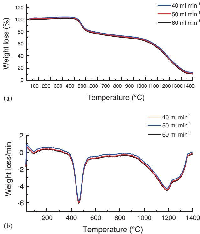
Figure 4. TGA-DTG plots of the Tirap coal sample at different flow rates (for external diffusion).
