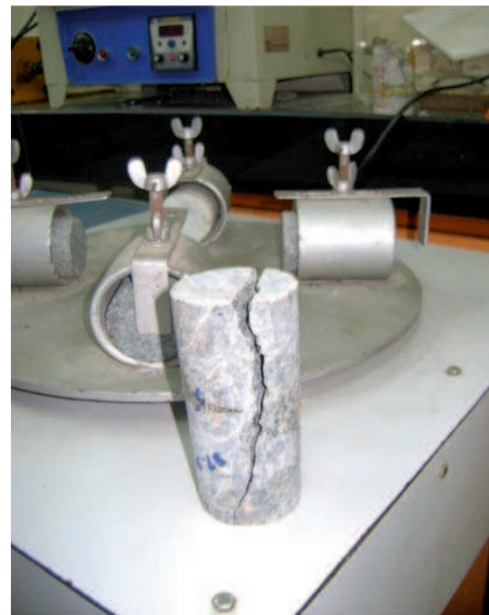
Figure 4. Fracture developed after UCS test.
