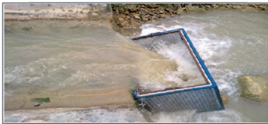
Figure 2. Bed load trap designed and constructed for the study.
