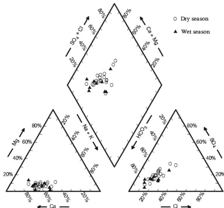
Figure 3. Piper trilinear diagram of the chemical types in groundwater of the study area.
