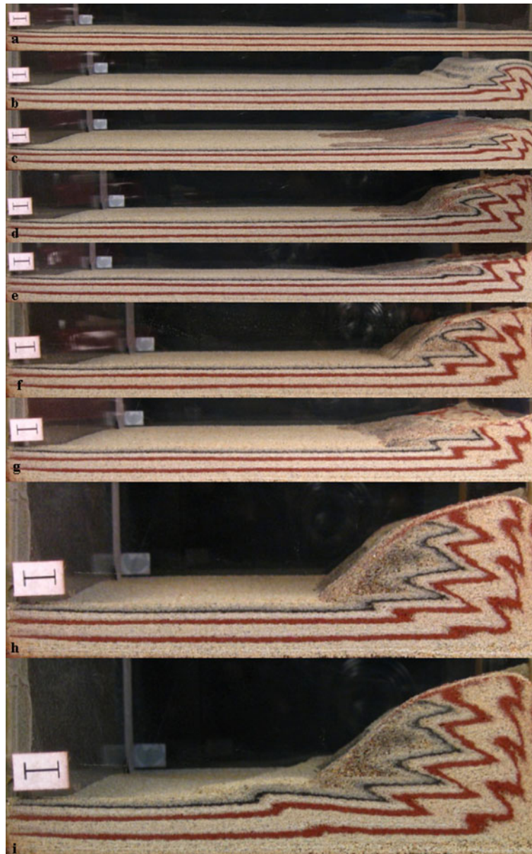
Figure 9(a). Abrupt increase in thrust spacing following cessation of surface erosion (see stage 'i' in the figure). Surface slope, \alpha = 0 and basal slope, \beta = 0 .
