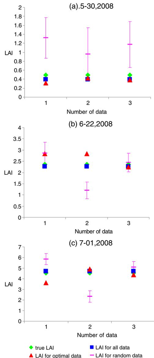
Figure 3. The comparison of field measured LAI with the inverted LAI for different data combination from field canopy reflectance measurement.
