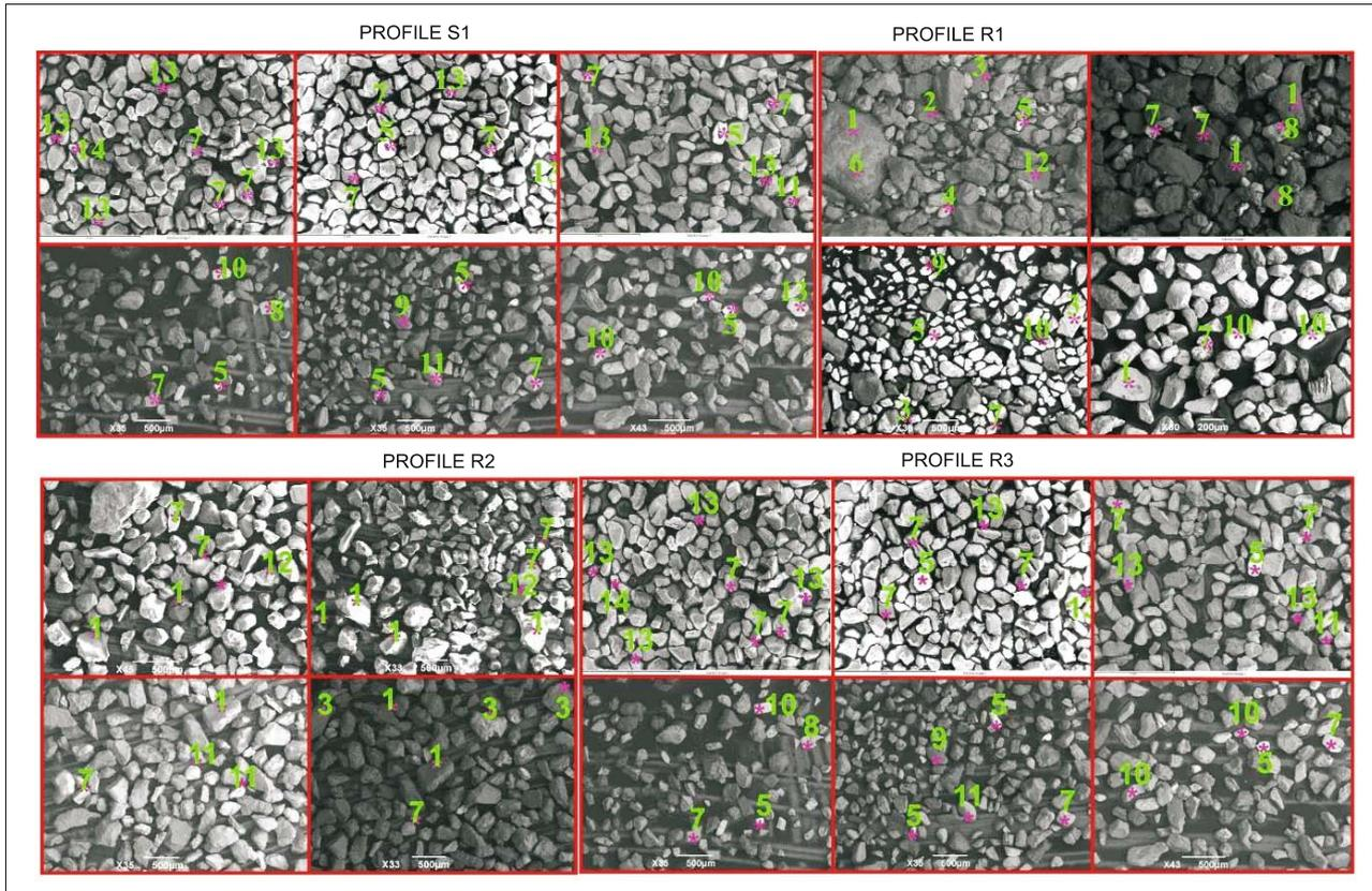
Figure 6. SEM microphotographs of the minerals that underwent high deformational episode with mineral names. 1. Quartz, 2. Calcic plagioclase, 3. K Feldspar, 4. Olivine, 5. Monazite, 6. Pyroxene, 7. Ilmenite, 8. Sphene, 9. Garnet, 10. Zircon, 11. Rutile, 12. Plagioclase feldspar, 13. Magnetite, and 14. Amphibole.
