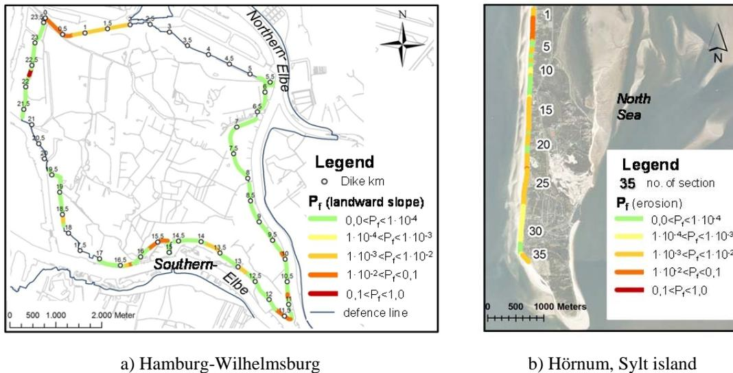
**Figure 7. Failure probabilities for the storm scenario XR2010A for a) dike breaches in Hamburg-Wilhelmsburg and b) dune erosion in Hörnum at the south end of Sylt island (after Naulin et al., 2012)**
