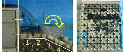
Figure 16. Experimental result, X-block, mass = 254 g
