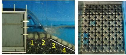
$h_1 = 5 \text{ cm}$  : Damaged
