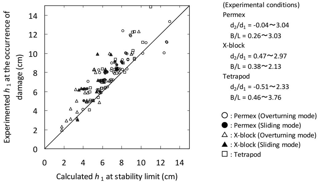
Figure 12. Calculated and experimented overflow depth of the stability limit.
