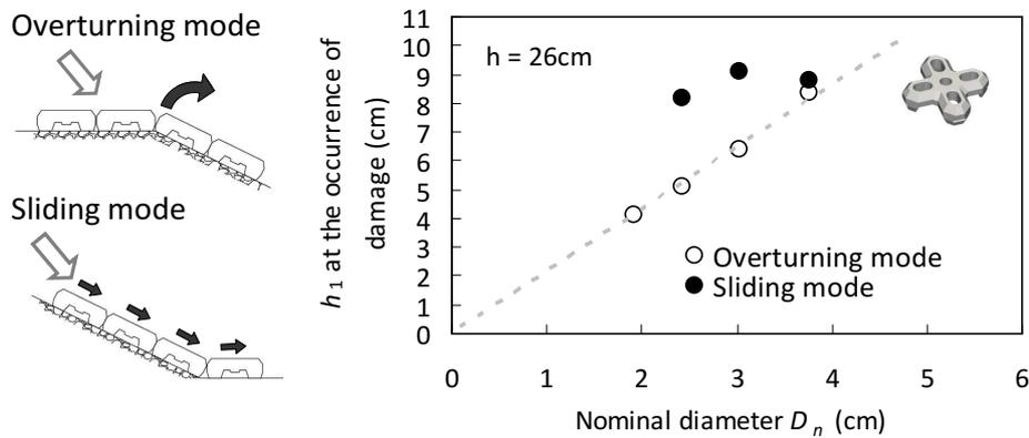
Figure 7. Relationship between the nominal diameter  $D_n$  and the overflow depth at the occurrence of damage by each failure mode.
