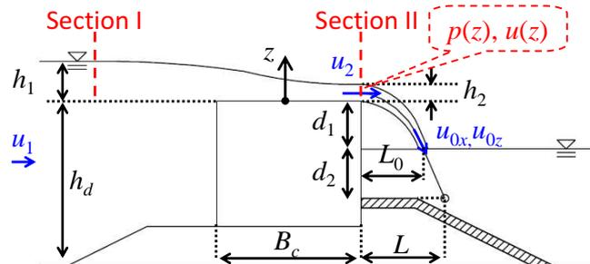
Figure 13. Definition of the symbols used in the calculation of the impingement position.
