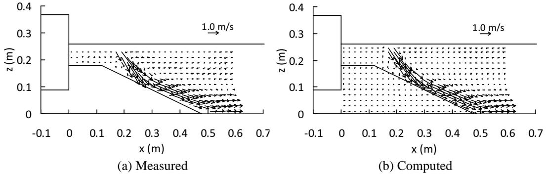
Figure 15. Comparison of measured and computed flow field,  $h_1 = 9$  cm.
