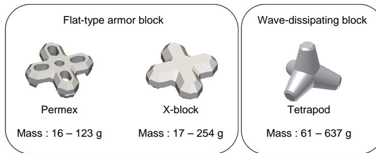
Figure 4. Armor units used in the experiments.
