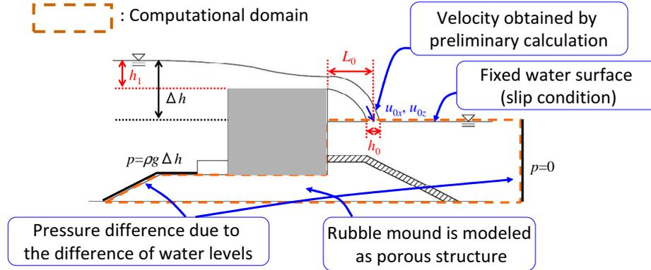
Figure 14. Schematic diagram of the computation method
