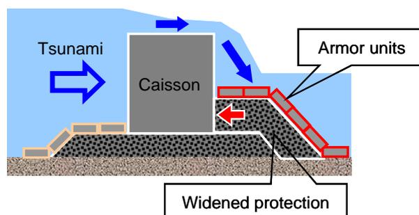
Figure 1. Countermeasure against tsunami of breakwaters.
