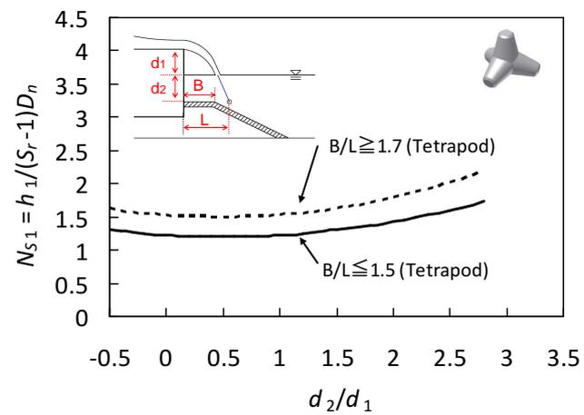
Figure 11. Stability numbers for wave-dissipating block.
