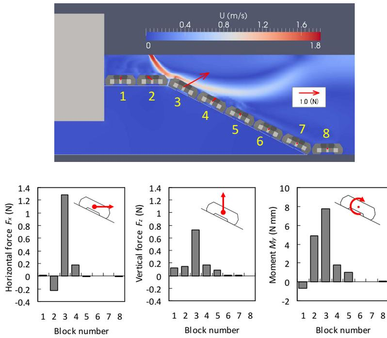
Figure 17. Computed flow field and fluid force acting on each block.
