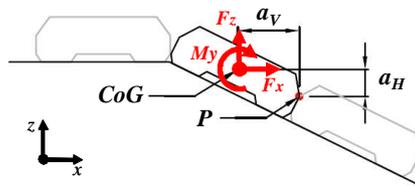
Figure 18. Analysis of the balance of moment of the block.
