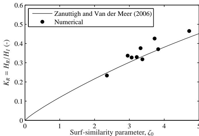
**Figure 5: Reflection coefficients for the Bilbao test case. Comparison with empirical relation presented in Zanuttigh and Van der Meer (2006)**
