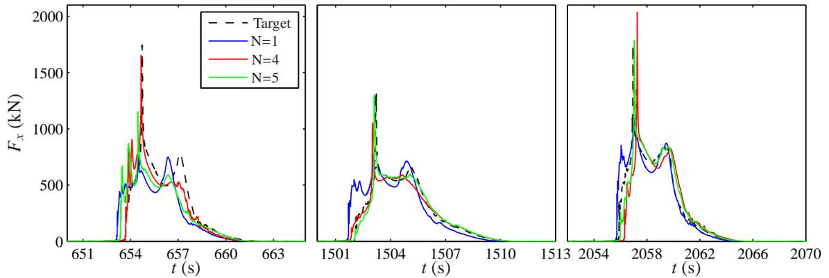
**Figure 9: Horizontal forces on the sea-wall of the breakwater for three impact events. The target represents the forces from the full irregular time series which is compared to the short reproductions.**
