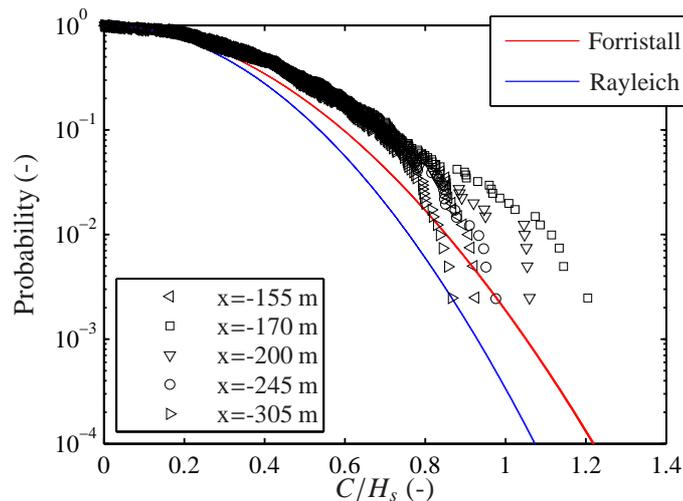
**Figure 1: Crest height,  $C$ , distribution for a significant wave height at  $H_s = 9.0$  m and a peak period at  $T_p = 11.0$  s. The  $x$ -values corresponds to the wave gauge position in the flume where  $x = 0$  is positioned 600 m from the inlet boundary.**
