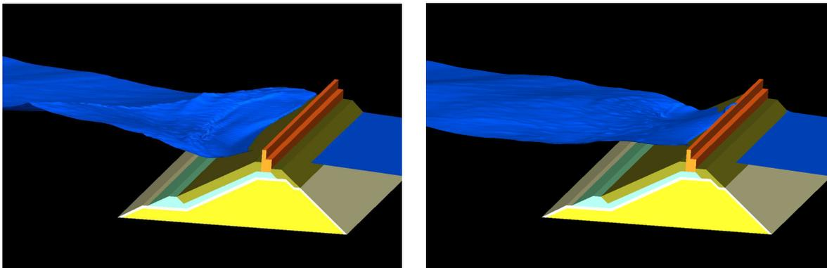
Figure 12: Visualization of the free surface during wave impact on the sea-wall.
