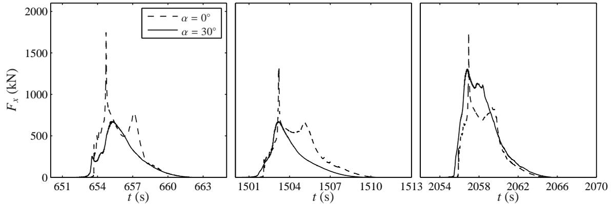
Figure 11: Effect of oblique waves on horizontal forces on the sea-wall of the breakwater.
