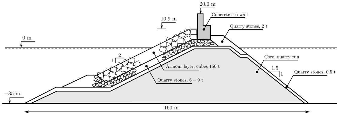
Figure 2: Sketch of the Bilbao breakwater profile. After Jensen (1984).
