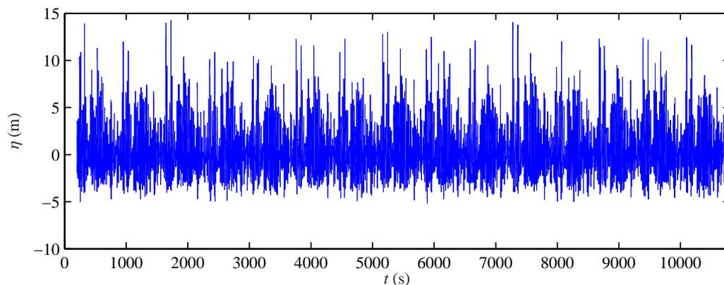
Figure 3: Surface elevation for the complete three hour irregular sea state for a significant wave height at  $H_s = 9.0$  m and a peak period at  $T_p = 15.0$  s.
