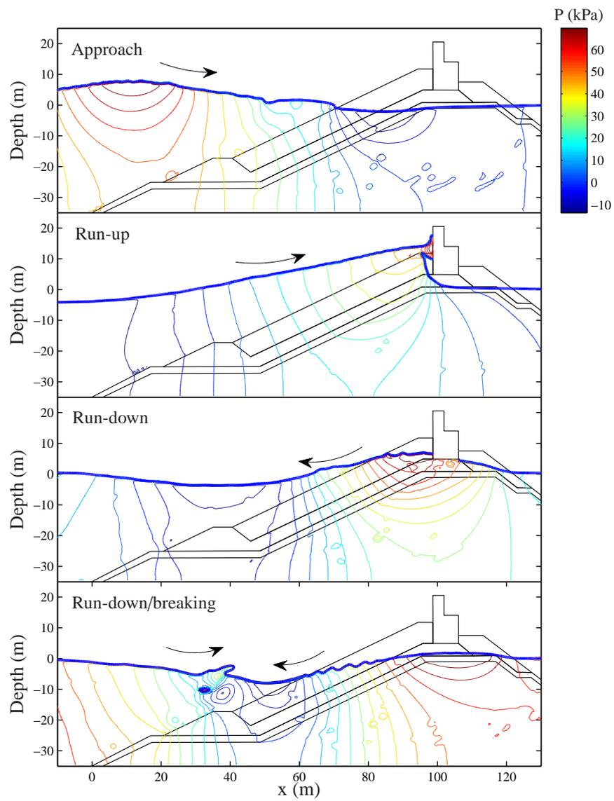
**Figure 7: Pressure contours for an impact event on the sea-wall represented by the approach, run-up and run-down stages.**
