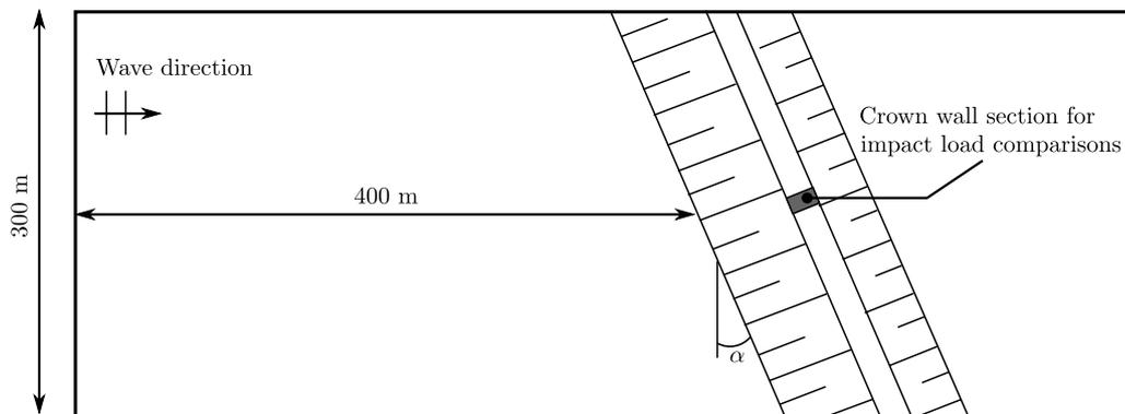
**Figure 10: Layout of the three-dimensional model domain for oblique wave interaction.**
