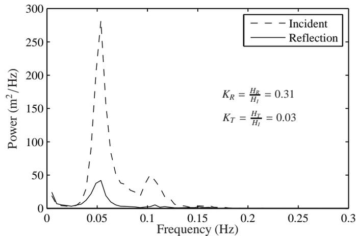
**Figure 4: Wave spectra for incident and reflected waves for an incident significant wave height at  $H_s = 10.0$  m and a peak period at  $T_p = 15.0$  s.**
