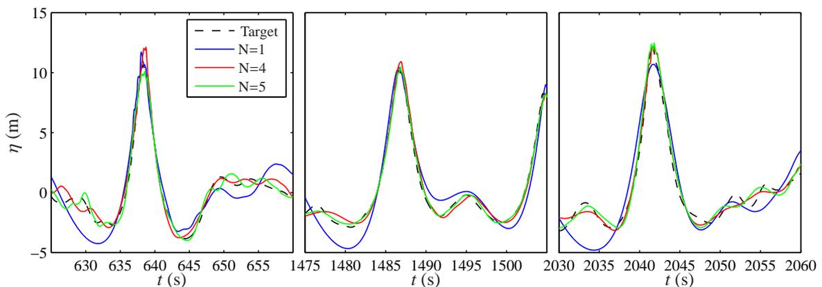
**Figure 8: Surface elevation in front of the breakwater for three impact events. The target represents the surface elevation from the full irregular time series which is compared to the short reproductions.**
