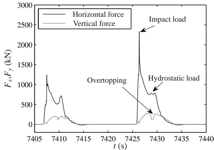
**Figure 6: Impact event on the breakwater sea-wall.**
