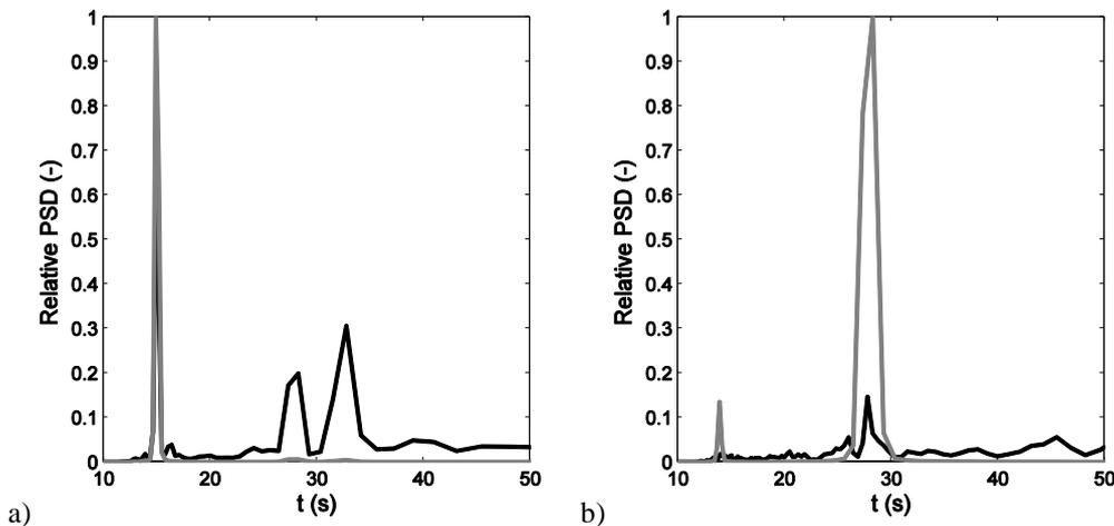
**Figure 7. Computed relative power spectral density of the computed bed level using the CCM<sup>+</sup> technique (black lines) and the band-pass filtered water surface elevation (grey lines) at the location  $x = 0.56-0.45$  m for case BE1 (a) and BE4 (b).**
