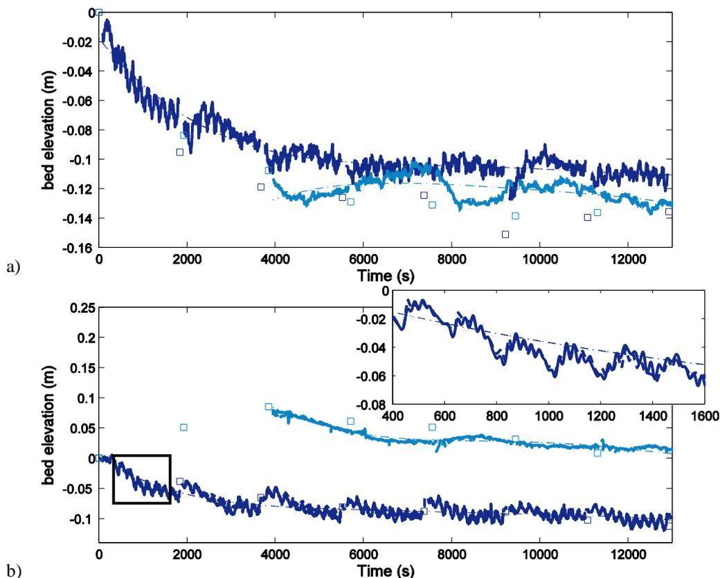
Figure 6. Time series of computed bed level from CCM<sup>+</sup> system (solid line), AWG (dotted line, plot a only) bottom profiler (squares), and trend line of CCM levels (dash-dotted line). Plot a: CCM tank 1 with cross-shore location  $x = 0.56$  m (BE1) and  $0.45$  m (BE4) Plot b: CCM tank 2 with cross-shore location  $x = 2.59$  m (BE1) and  $2.48$  m (BE4). Darker lines correspond to BE1 case while lighter lines correspond to case BE4
