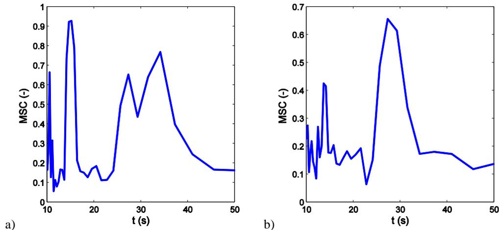
Figure 8. Computed magnitude-squared coherence (MSC) between the computed bed level using the CCM<sup>+</sup> technique and the band-pass filtered water surface elevation at the location  $x = 0.56-0.45$  m for case BE1 (a) and BE4 (b).
