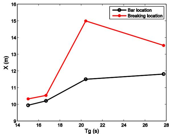
Figure 4. Cross-shore bar and wave breaking locations as a function of wave group period.
