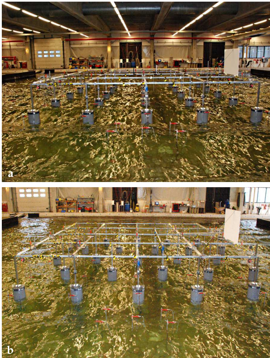
Figure 2. The 5x5-WEC rectilinear (a) and staggered (b) farm in the DHI Shallow Water Wave Basin under irregular long-crested waves with \theta = 0^\circ . View from behind the wave generator.
