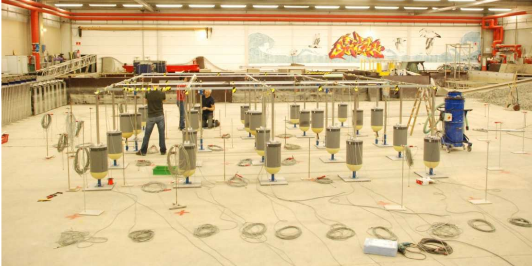
Figure 3. Construction of WEC support structures in the DHI wave basin.
