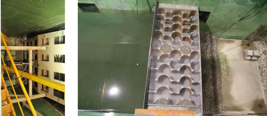
Figure 6. Absence of water leakages: a) wave paddle with interior face completely dry (left), b) model of the *cyes-R* with water on the left and dry (right).
