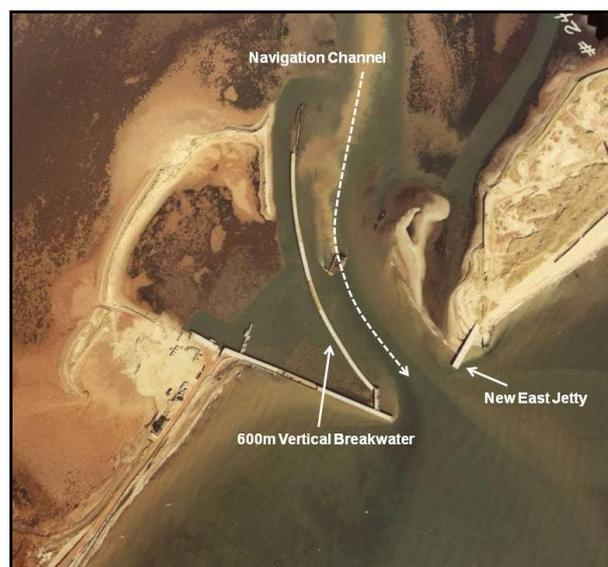
**Figure 3. Aerial photograph taken in 1980 showing coastal works constructed during the late 1960's and early 1970's (PWGSC, 1980, with permission from Public Works and Government Services Canada).**
