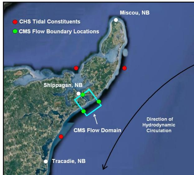
**Figure 6.** A regional tidal model was developed and applied to predict the tidal fluctuations at three locations corresponding to the boundaries of the CMS-Flow domain (pictured). Model input was based on tidal constituent data obtained from CHS (Google Earth, 2011).
