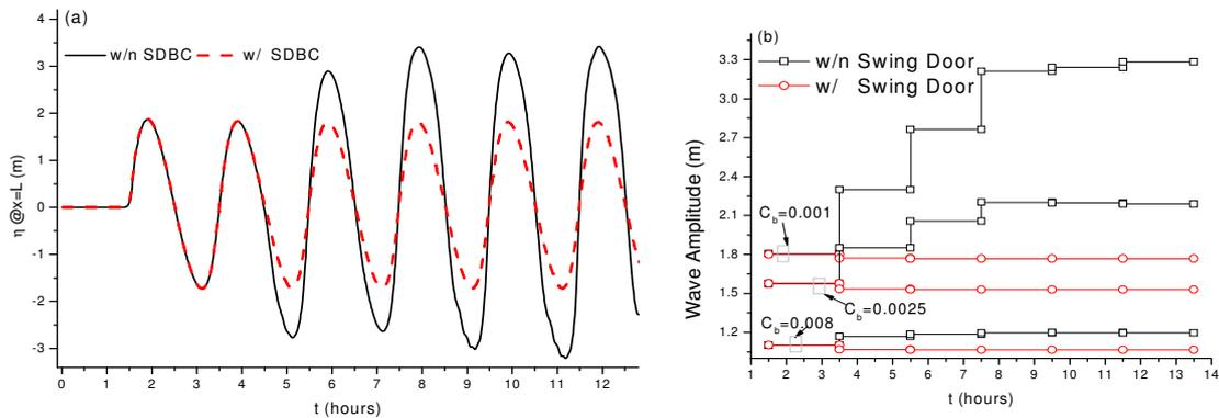
**Figure 7 Tests on Swing-Door Boundary Condition in a channel with length of  $L = 0.75\lambda$ . (a) Time series of elevation at  $x=L$  for small friction condition,  $C_b = 0.001$ ; (b) Variation of elevation amplitude at  $x=L$  for various friction conditions.**
