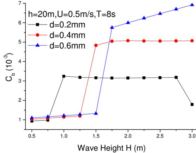
Figure 1 Bottom friction factor in typical coastal conditions
