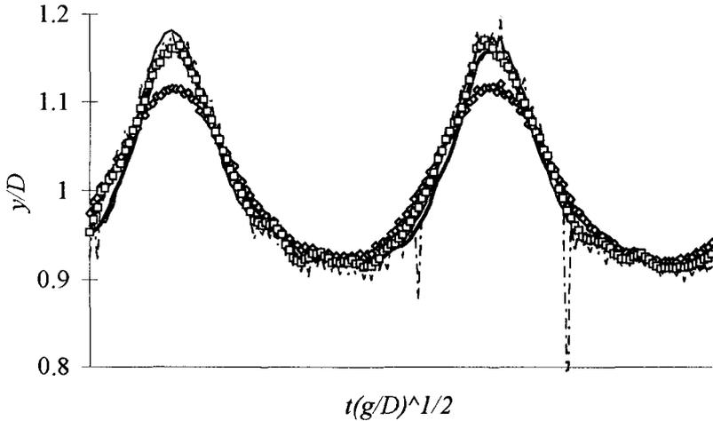
Figure 8: regular wave,  $T = 4.1\text{s}$ ,  $y_p/D = 0$ ,  $c_s = 0$ ,  $\lambda/D \approx 12$
