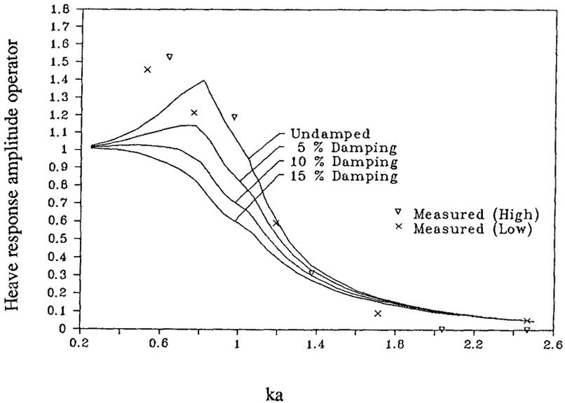
Fig. 7. Numerical and laboratory results of the heave response amplitude operator for the rectangular breakwater.
