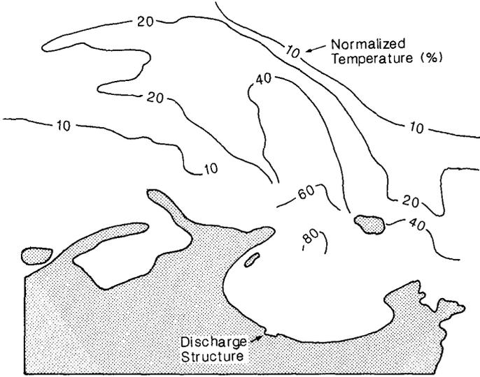
Figure 19a. Offshore Plume Configuration for Model Test 6-3 027
