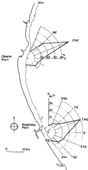
Figure 5 Wave directions at Oharai and Kashima Ports.
