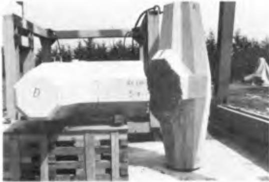
Photograph 5: The breakage of Dolos (Drop test)
