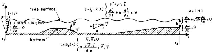
Figure 1 - Boundary conditions - Left b.c. simulates a wave-machine (e.g.  $U = U_0(z) \sin \omega t$ ) - Right b.c. is absorbing if  $h$  is small enough to eliminate dispersive phenomena. On the bottom, the second b.c. simulates a tangential stress in a boundary layer.
