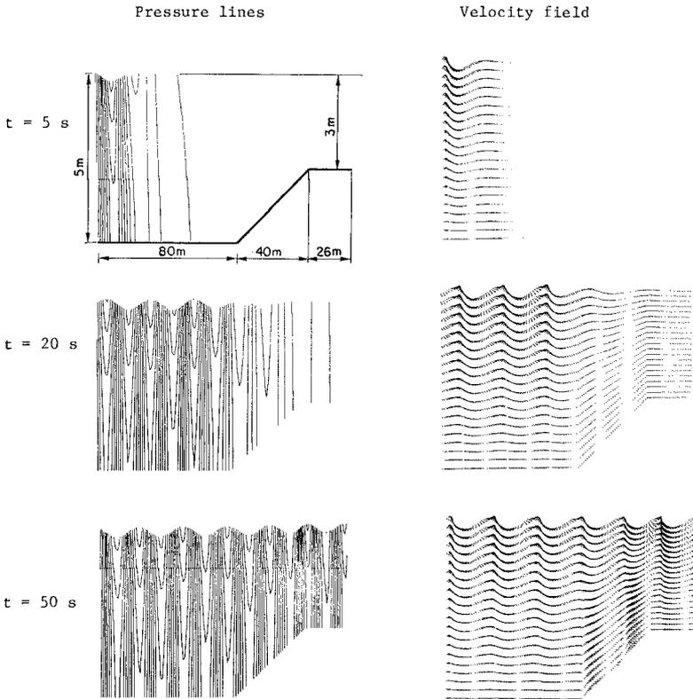
Figure 4 - Waves calculated in the numerical wave flume.
