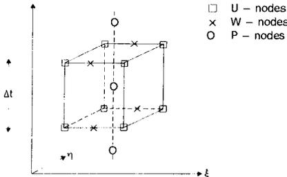
Figure 3 - Numerical staggered grid, in space and time.
