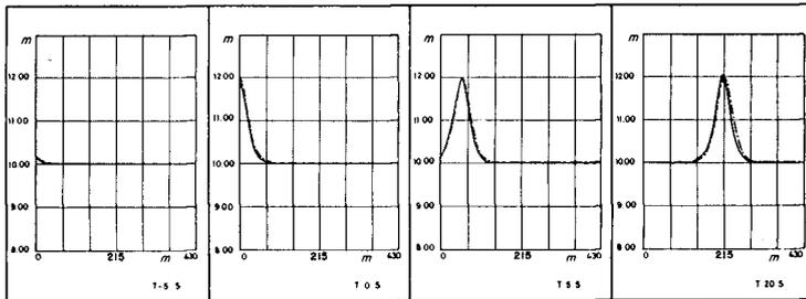
Figure 5 - Free surface of a solitary wave at  $t = -5$  s, 0 s, 5 s, 20 s.
