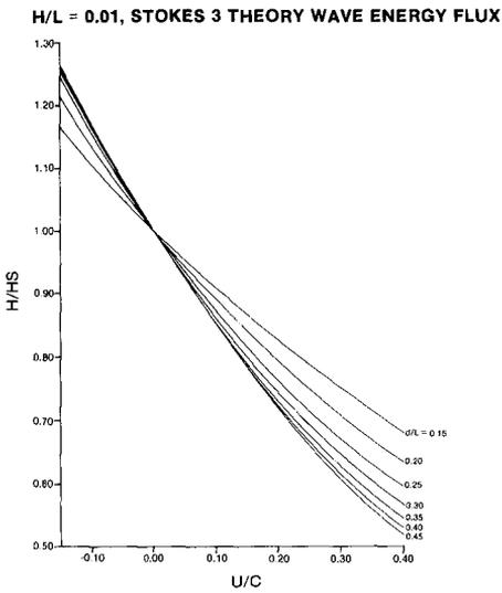
Fig. 5. The wave height change by Stokes (3rd) third-order wave theory for  $H_S/L_S=0.01$
