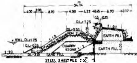
FIG. 22. - CROSS-SECTION OF THE SEA-WALL OF THE KANSAI ELECTRIC POWER CO.LTD
