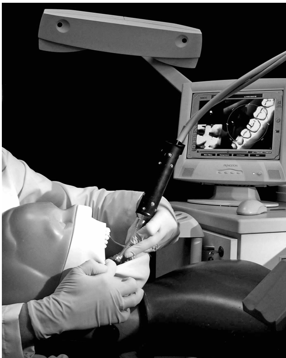
Figure 2. How the computerized dental simulator (DentSim) combines a patient mannequin, rotary instruments, and a computer monitor with real-time feedback
