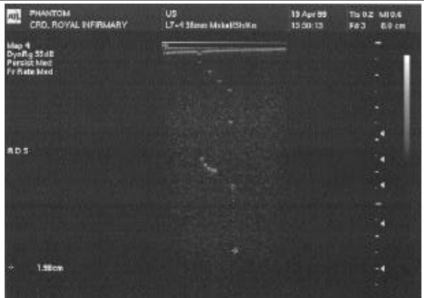
Fig. 3. Phantom. The crosses mark the position of the wire markers and the dotted line is the distance between the two markers.
