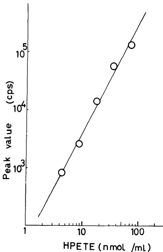
Fig.1. Chemiluminescent intensity (counts at peak) against concentration in the assay of HPETE with luminol-CHP. The concentrations of luminol and CHP were as indicated in section 2. The concentration of HPETE was determined independently by iodometries.
