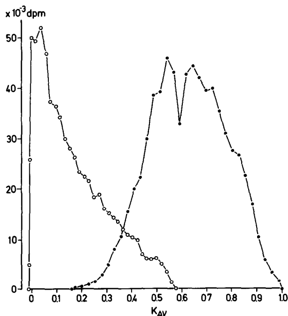
Fig.6. ^3\text{H} -Labelled HS-chains were chromatographed on a 1.1 \times 96 cm column of AcA 44 ( \circ-\circ ), and on a 1.1 \times 90 cm column of Sepharose 4B ( \bullet-\bullet ). Chromatographic conditions as in fig.4.
