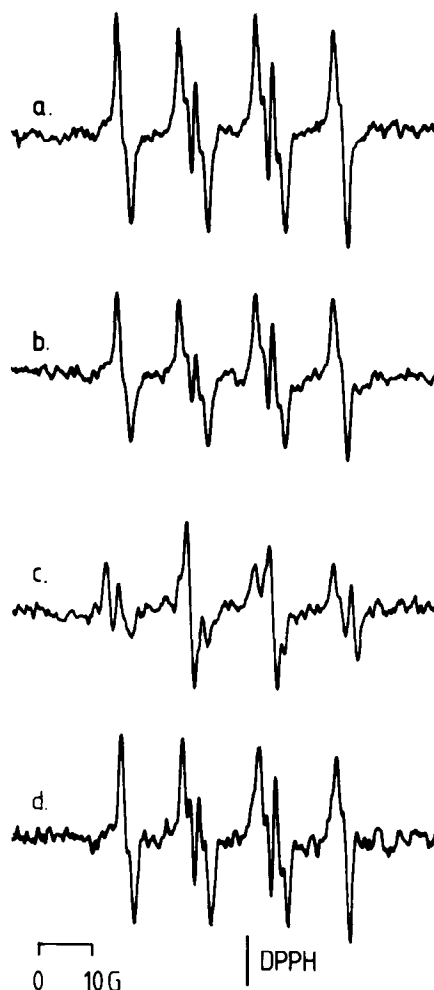
Fig. 1. Spin trapping of oxygen-centred radical, in the presence of 100 mM DMPO, produced by: (a) NADPH oxidase 20 \mu g/ml; (b) NADPH oxidase/50 \mu M transferrin; (c) NADPH oxidase/100 \mu M transferrin/178 \mu M H_2O_2 ; (d) NADPH oxidase/80 \mu M myeloperoxidase/178 \mu M H_2O_2 . All reaction mixtures contained 1 mM NADPH.
