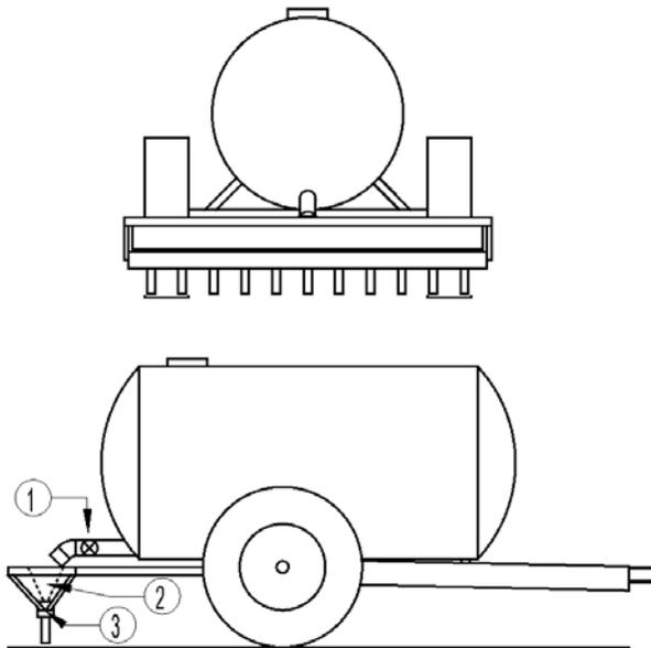
**Fig. 1. Configuration of the plot manure spreader showing distribution of drop tubes and (1) location of ball valve, (2) upper distribution trough, and (3) lower distribution trough.**
