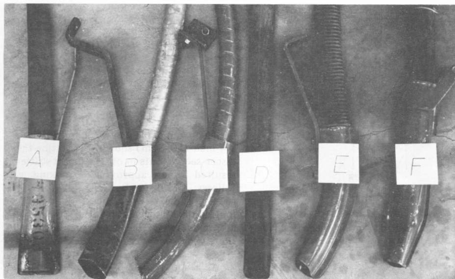
Figure 4. Discer seed spouts evaluated.
