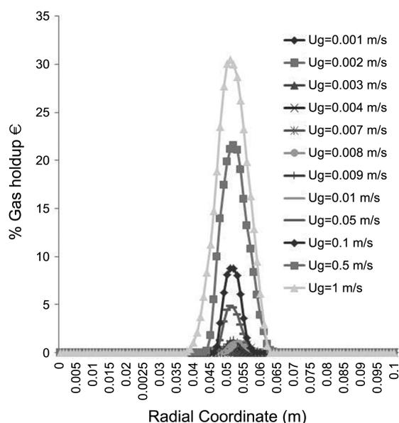
**Figure 3.** Radial distribution of gas holdup. Values measured at a height of 0.5 m from the gas distributor.
