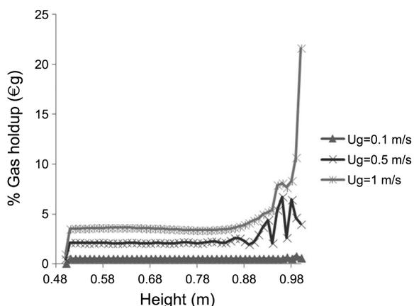
**Figure 5.** Gas Holdup Distribution along Column Height, values measured from a height of 0.5 m from gas distributor (For higher gas velocities).
