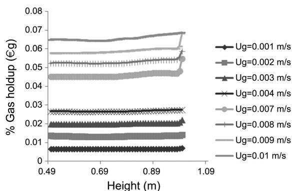
**Figure 4.** Gas Holdup Distribution along Column Height, values measured from a height of 0.5 m from gas distributor (For lower gas velocities).
