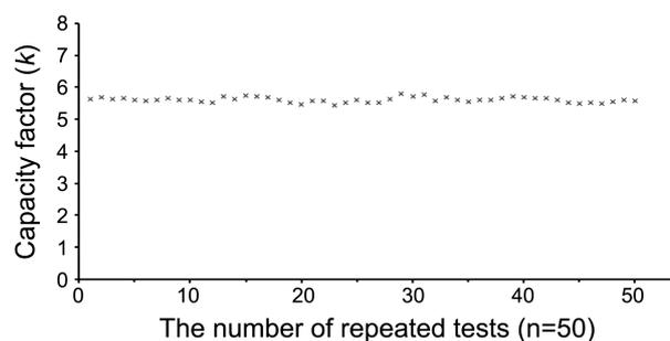
**Figure 6.** Dependence of capacity factors ( $k$ ) of thiamine versus the number of repeated tests ( $n = 50$ ) using aqueous 10 mmol/L ammonium formate (pH 3.5) with 30 mmol/L [EMIM][PF<sub>6</sub>] as a mobile phase.**Table 4.** Comparison of the proposed method with the current official method
