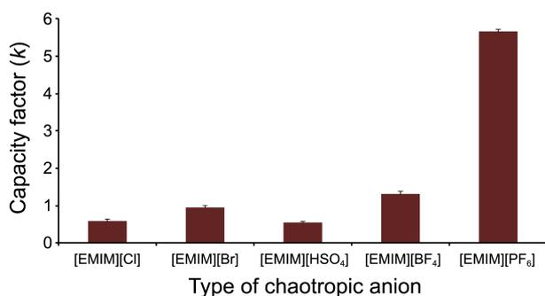
**Figure 2.** Effect of chaotropic anion type on the capacity factors ( $k$ ) of thiamine. Mobile phase: 10 mmol/L ammonium formate (pH 3.5) with the addition of different 30 mmol/L [EMIM]-based RTILs.
