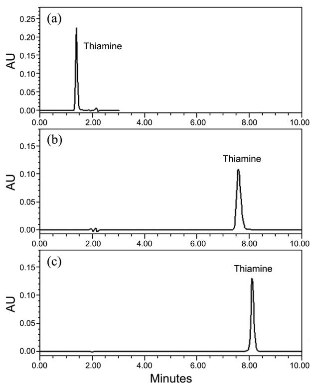
**Figure 7.** Chromatograms of thiamine with (a) an aqueous mobile phase without [EMIM][PF<sub>6</sub>], (b) an organic mobile phase containing sodium 1-octanesulfonate (current official method) and (c) an aqueous mobile phase containing 30 mmol/L [EMIM][PF<sub>6</sub>] (proposed method).
