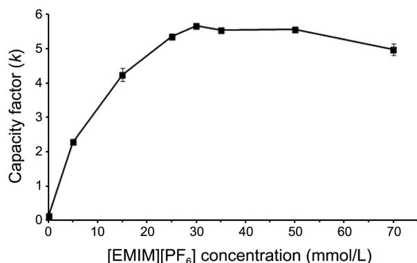
**Figure 4.** Effect of [EMIM][PF<sub>6</sub>] concentration on the capacity factors ( $k$ ) of thiamine. Mobile phase: 10 mmol/L ammonium formate (pH 3.5) with different concentrations of [EMIM][PF<sub>6</sub>].
