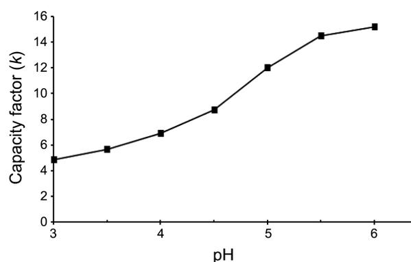
**Figure 5.** Effect of mobile phase pH on the capacity factors ( $k$ ) of thiamine. Mobile phase: 10 mmol/L ammonium formate (pH 3.0 to 6.0) with 30 mmol/L [EMIM][PF<sub>6</sub>].
