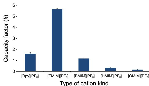
**Figure 3.** Effect of cation type on the capacity factors ( $k$ ) of thiamine. Mobile phase: 10 mmol/L ammonium formate (pH 3.5) with the addition of different 30 mmol/L [PF<sub>6</sub>]-based RTILs. Methanol was added into the mobile phase when [HMIM][PF<sub>6</sub>] and [OMIM][PF<sub>6</sub>] were used as mobile phase additives.
