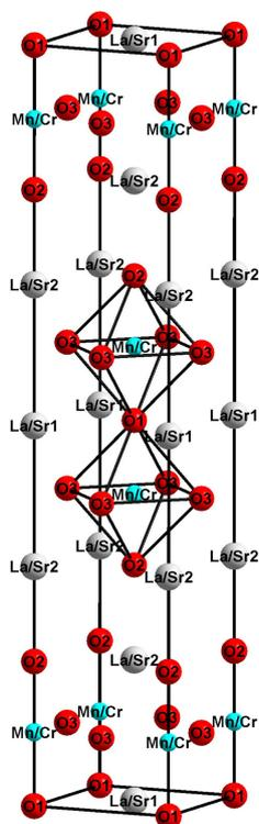
**Figure 3.** Unit cell structure of  $\text{LaSr}_2\text{MnCrO}_7$ .
