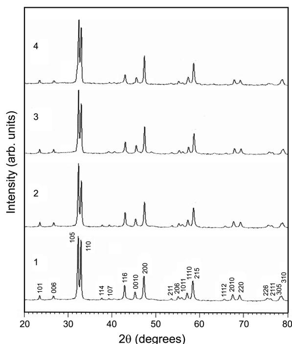
**Figure 1.** X-ray powder diffraction patterns of  $\text{LaSr}_2\text{MnCrO}_7$ (1),  $\text{La}_{0.8}\text{Nd}_{0.2}\text{Sr}_2\text{MnCrO}_7$ (2),  $\text{La}_{0.8}\text{Gd}_{0.2}\text{Sr}_2\text{MnCrO}_7$ (3), and  $\text{La}_{0.8}\text{Dy}_{0.2}\text{Sr}_2\text{MnCrO}_7$ (4).
