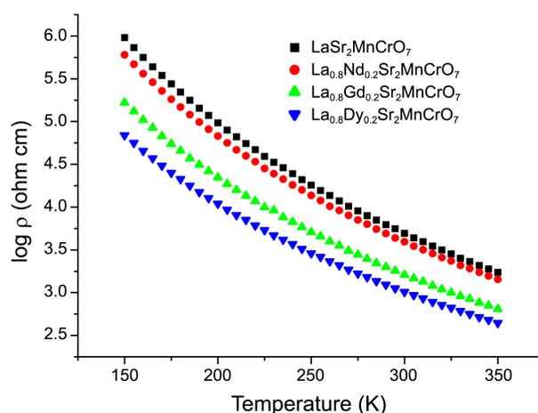
**Figure 5.** Plots of  $\log \rho$  versus Temperature (K) of  $\text{LaSr}_2\text{MnCrO}_7$ ,  $\text{La}_{0.8}\text{Nd}_{0.2}\text{Sr}_2\text{MnCrO}_7$ ,  $\text{La}_{0.8}\text{Gd}_{0.2}\text{Sr}_2\text{MnCrO}_7$ , and  $\text{La}_{0.8}\text{Dy}_{0.2}\text{Sr}_2\text{MnCrO}_7$ .
