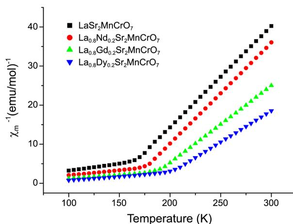
**Figure 4.** Plots of inverse molar magnetic susceptibility ( $\chi_m^{-1}$ ) versus Temperature (K) of  $\text{LaSr}_2\text{MnCrO}_7$ ,  $\text{La}_{0.8}\text{Nd}_{0.2}\text{Sr}_2\text{MnCrO}_7$ ,  $\text{La}_{0.8}\text{Gd}_{0.2}\text{Sr}_2\text{MnCrO}_7$ , and  $\text{La}_{0.8}\text{Dy}_{0.2}\text{Sr}_2\text{MnCrO}_7$ .
