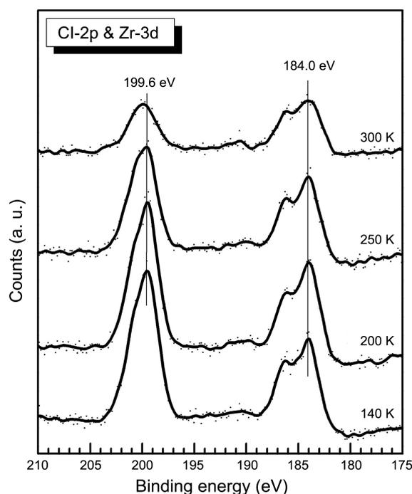
**Figure 2.** The Cl 2p and Zr 3d XPS features of ZrCl<sub>4</sub> adsorbed on the OH/SiO<sub>2</sub>/Si(111) surface. The surface was prepared by dosing 100 L of ZrCl<sub>4</sub> at 140 K and heated to the indicated temperatures.
