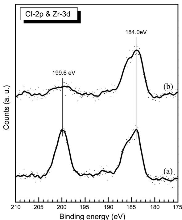
**Figure 3.** Change of Cl 2p and Zr 3d XPS features of ZrCl<sub>2</sub> species produced on the OH/SiO<sub>2</sub>/Si(111) surface. The surfaces were prepared as follows: (a) The surface covered with ZrCl<sub>4</sub> was heated to 300 K to produce ZrCl<sub>2</sub> species. (b) The surface (a) was exposed to H<sub>2</sub>O at 300 K followed by heating to 600 K.
