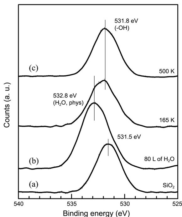
**Figure 1.** Oxygen 1s XPS features after treating the Si (111) surface with O<sub>2</sub> and H<sub>2</sub>O. (a) The Si(111) surface was heated at 1090 K for 30 min in  $1.0 \times 10^{-4}$  torr of O<sub>2</sub>. (b) The surface (a) was exposed to 80 L of H<sub>2</sub>O at 140 K. (c) The surface (b) was heated to 500 K.
