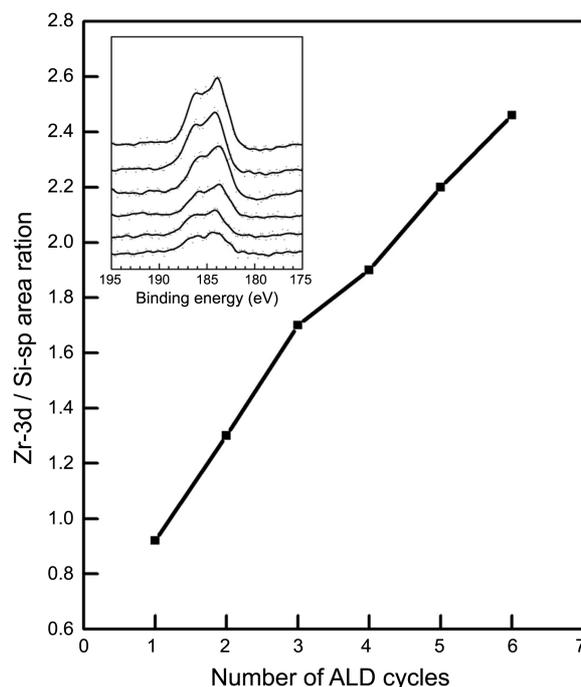
**Figure 4.** The XPS peak area ratio of Zr 3d to Si 2p. One ALD cycle is completed by ZrCl<sub>4</sub> dosing at 140 K, heating to 550 K, H<sub>2</sub>O dosing at 300 K, and heating to 600 K. The insert figure shows XPS features of ZrO<sub>2</sub> after each cycle.
